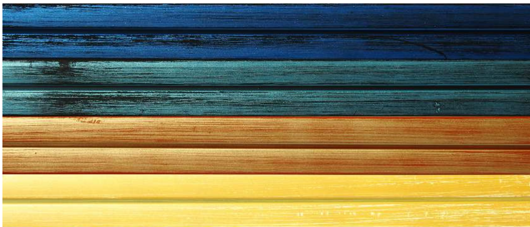
From the top: ASM 700 blue pearl patina applied on a black primer, then sanded; ASM 600 green pearl patina applied on a black primer, then sanded; ASM 459 gold pearl patina applied on a red primer, then sanded; ASM 200 yellow pearl patina applied on a white primer, then sanded.
