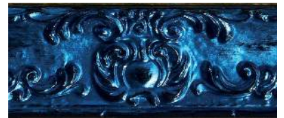
Moulding varnished with ASM 700 alcohol-based blue-pearl patina on black base, then sanded.
