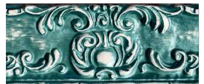
Moulding varnished with ASM 600 alcohol-based green-pearl patina on white base, then sanded.
