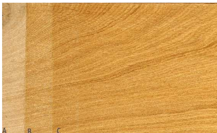
Section A: Rough wood. Section B: 1 coat of PRW 900. Section C: 2 coats of PRW 900.
